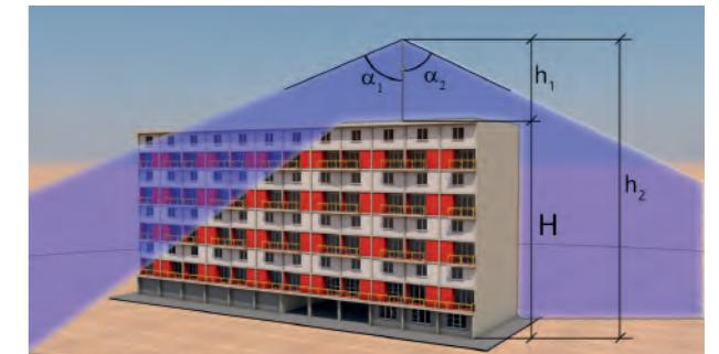
Fig. 7 – Protection volume angles  $\alpha_1$  and  $\alpha_2$  depending on heights  $h_1$  and  $h_2$ .
