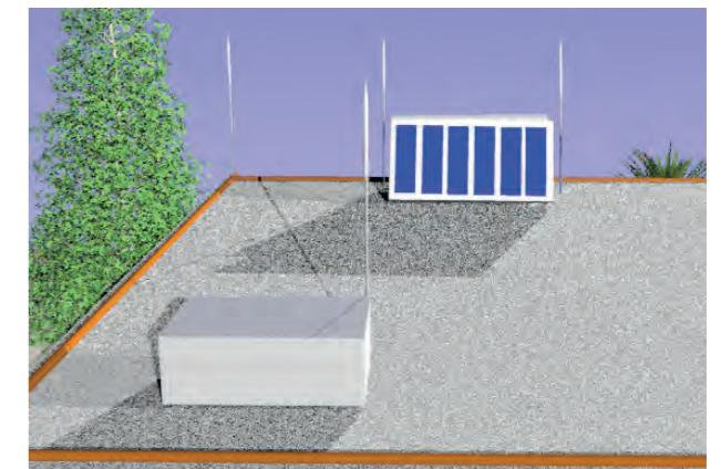
Fig. 10 – Protection of protruding structures with a capture mesh system by lightning rods.
