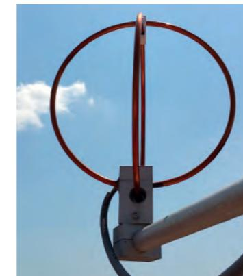
Fig. 24 – LINET field antenna sensor.
