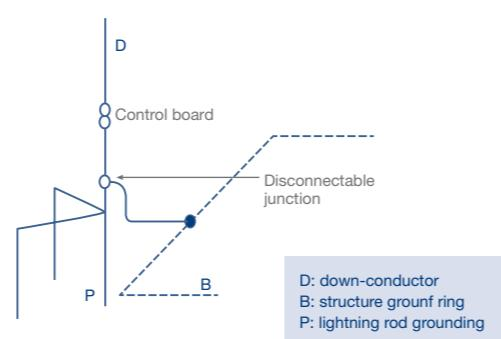
Fig. 16 – Example of grounding of type A2. The stakes will be linked by a conductor with the same characteristics and section of the down-conductor.
