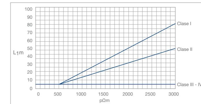
Fig. 18. – Minimum lenght (L1) of each ground electrode according to the class of LPS.
