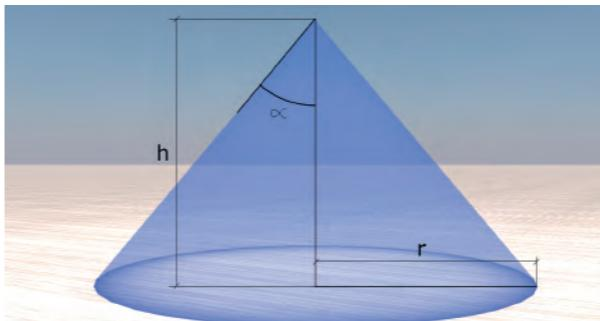
Fig. 6 – Protected volume by a vertical point. IEC 62305-3.
