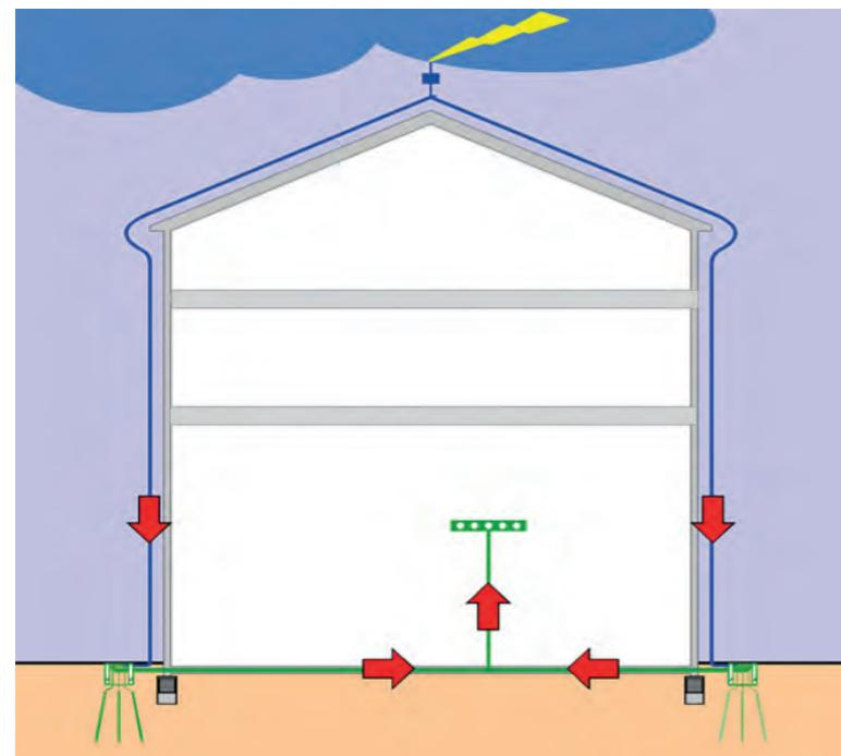
Fig. 11 – Down conductors of LPS by ESE.
