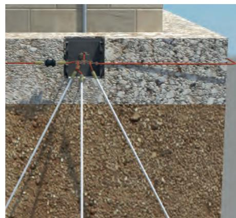
Fig. 13 – Grounding System cross section.
