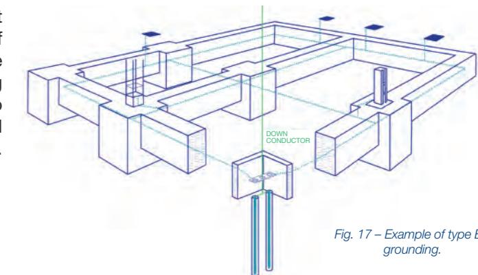
Fig. 17 – Example of type B grounding.
