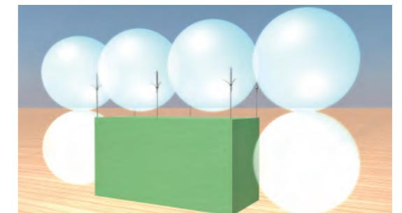
Fig. 8 – Protected volume by the rolling sphere method.
