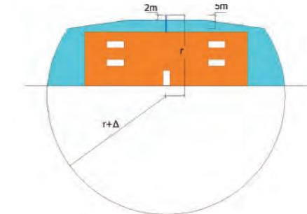
Fig. 3 – Volume protected with ESE lightning rod.
