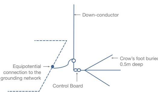
Fig. 15 – Example of grounding of type A1: 3 horizontal conductors (deep: 50cm, length: 7 to 8m).
